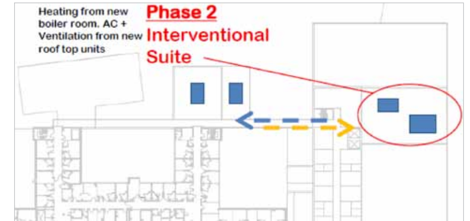
Figure 5 – CSA Class 1 compliant AHUs to serve the Interventional Suite
