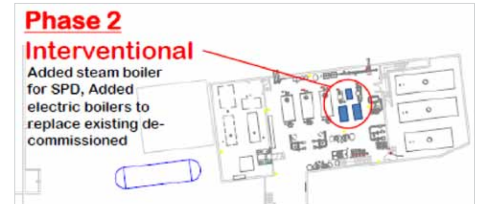
Figure 6 – Existing Energy Centre
